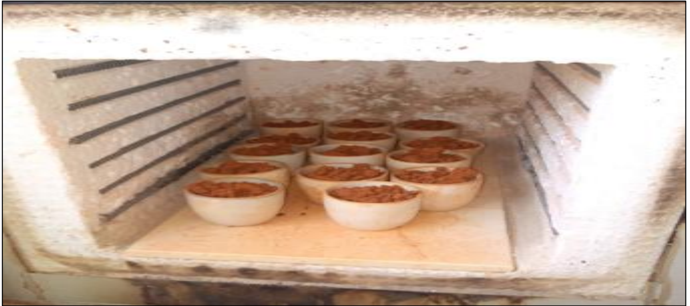
Fig 1 Calcined Clay Soil in a Furnace.
