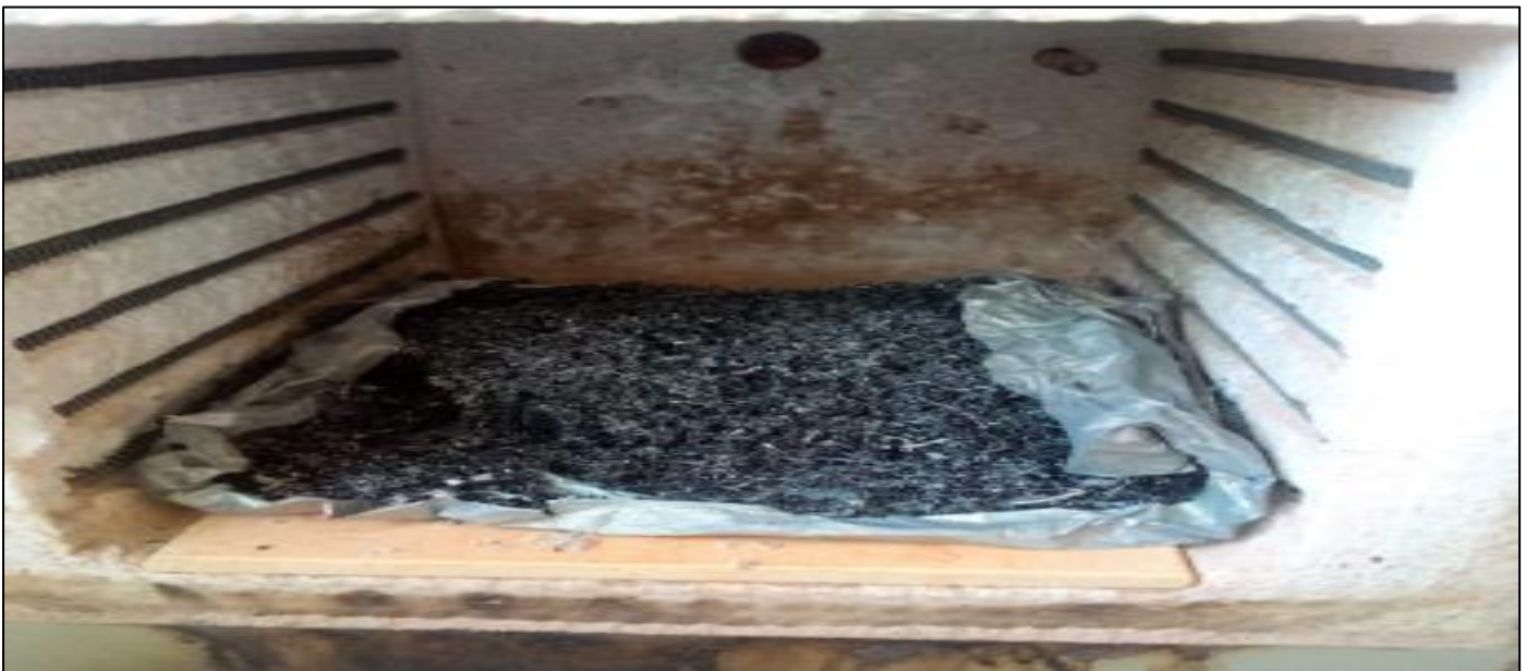
Fig 2 Calcined Sorghum Husks in a Furnace.
