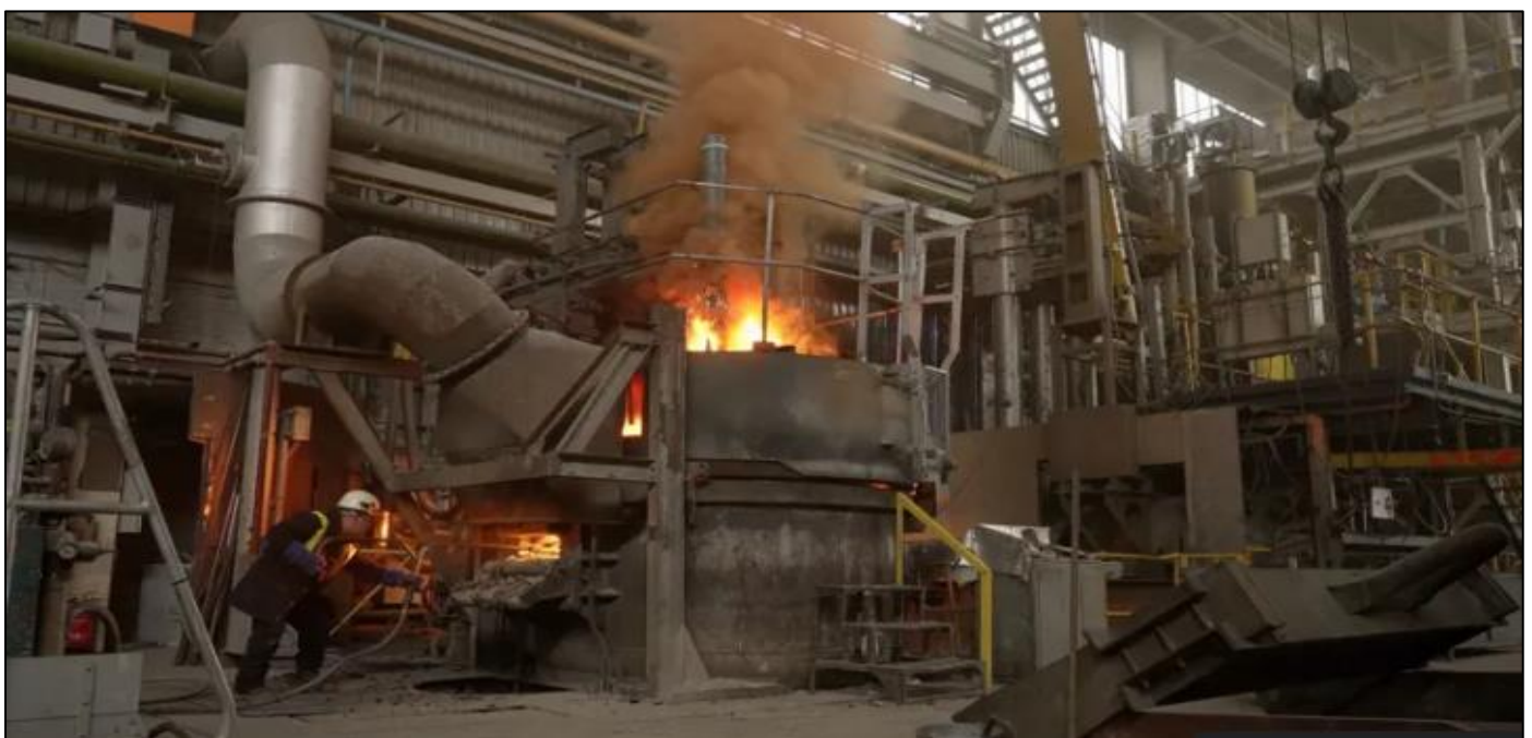
Fig 7 Flames Emerge from the Top of an Arc Furnace as the Material that will form the Slag is Added to the Molten Steel
