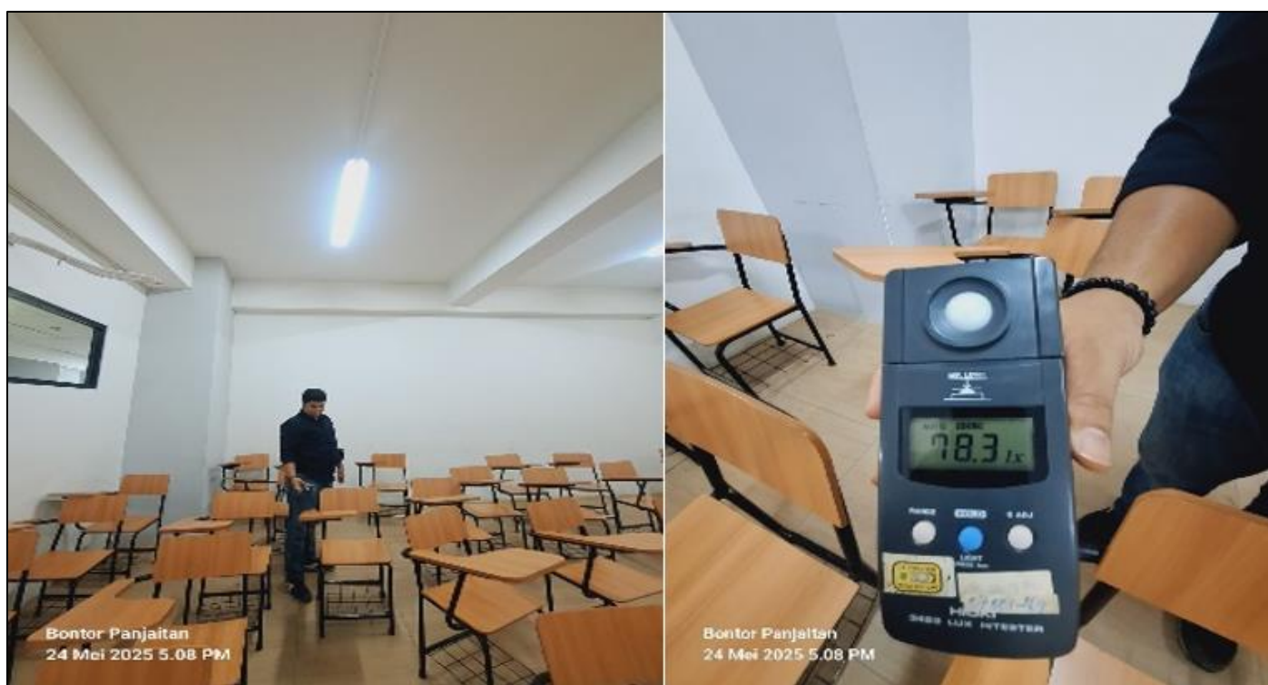
Fig 3 Actual Lighting Measurement with Hioki-3432 Measuring Device
