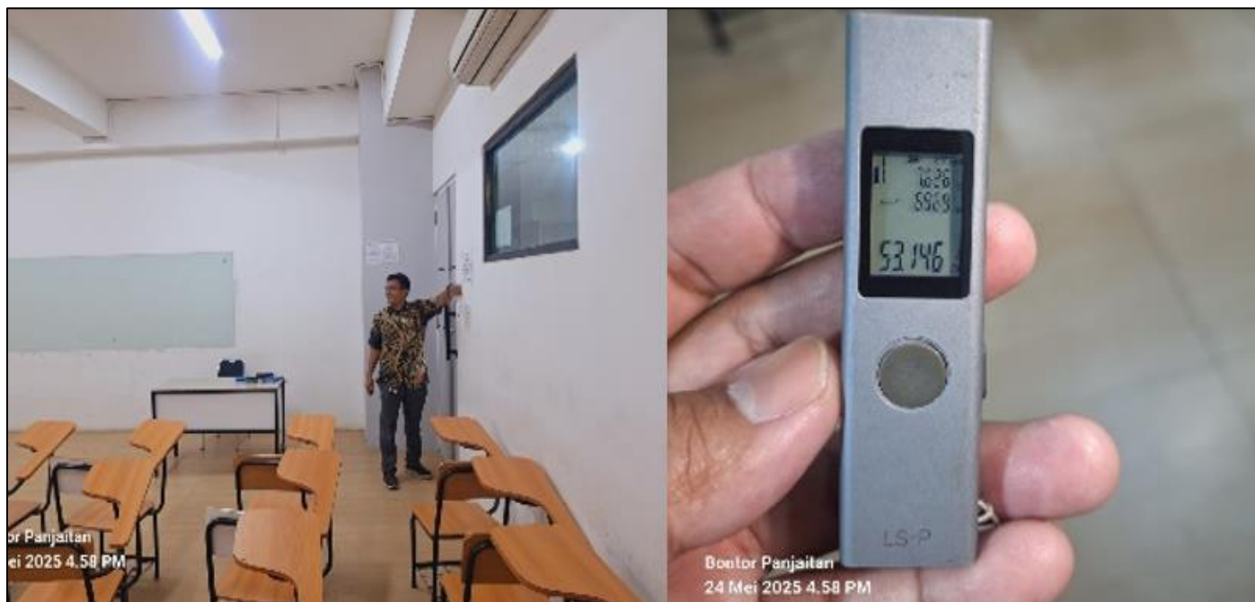
Fig 2 Actual Measurement of Classroom Area and Height.
