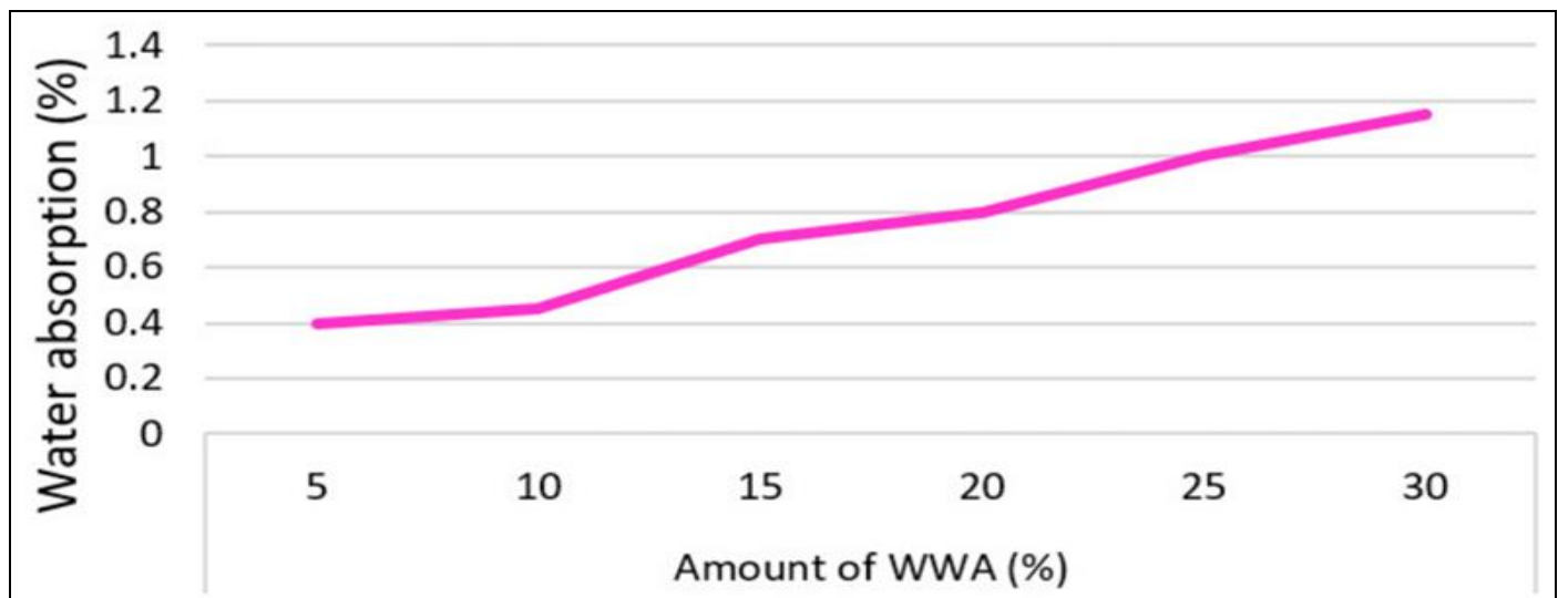
Fig 1 Percentage of Water Absorption Versus Ash Content of WWA Concrete. [25]
