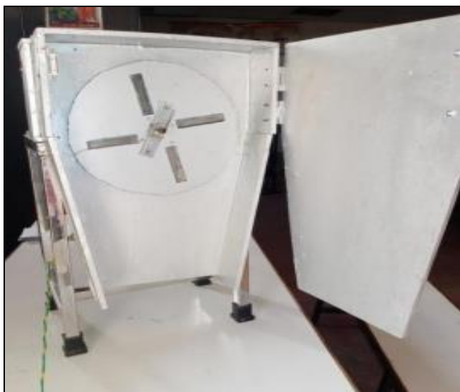
Fig 4 Blade Arrangement of Vegetable Slicer
