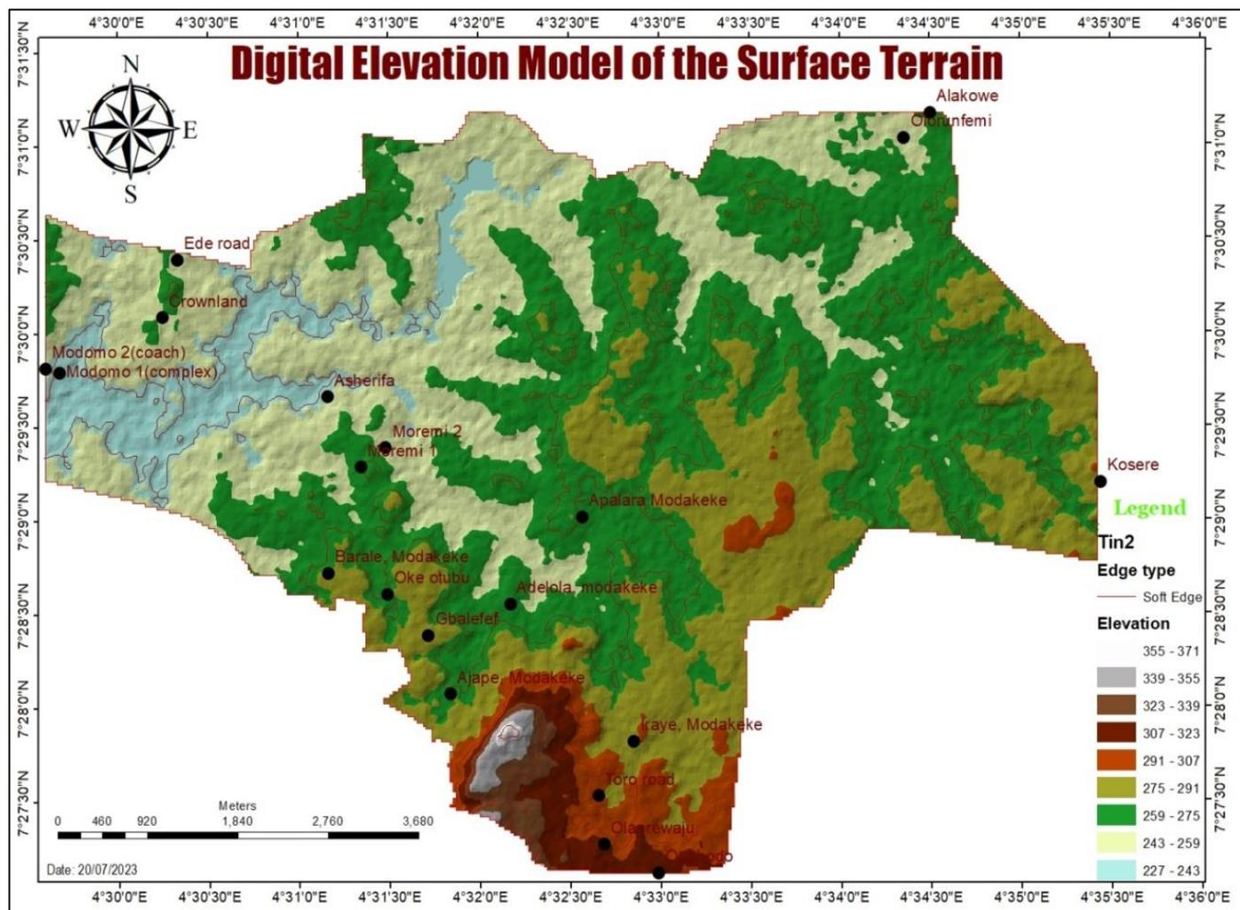
Fig 6 Showing Digital Elevation Model of Surface Terrain or Surface Configuration
