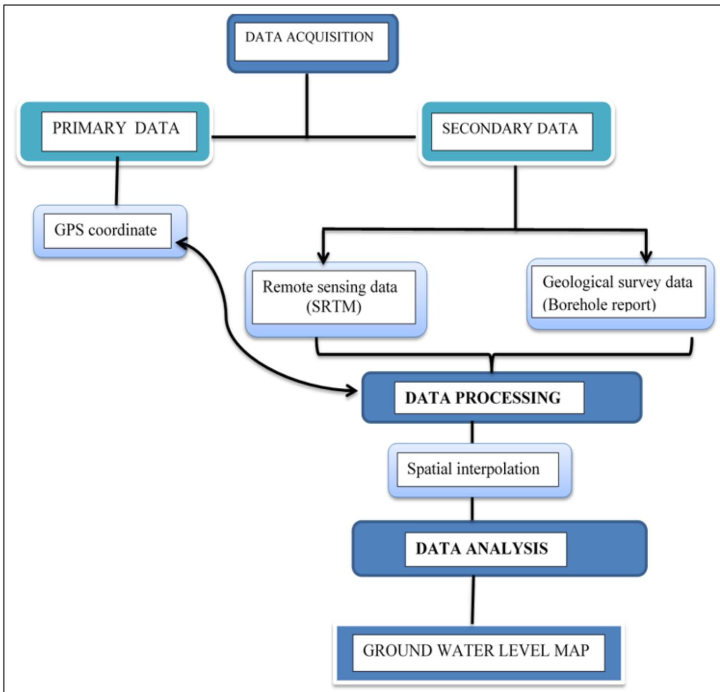
Fig 1 Showing Water Level Mapping Procedure
