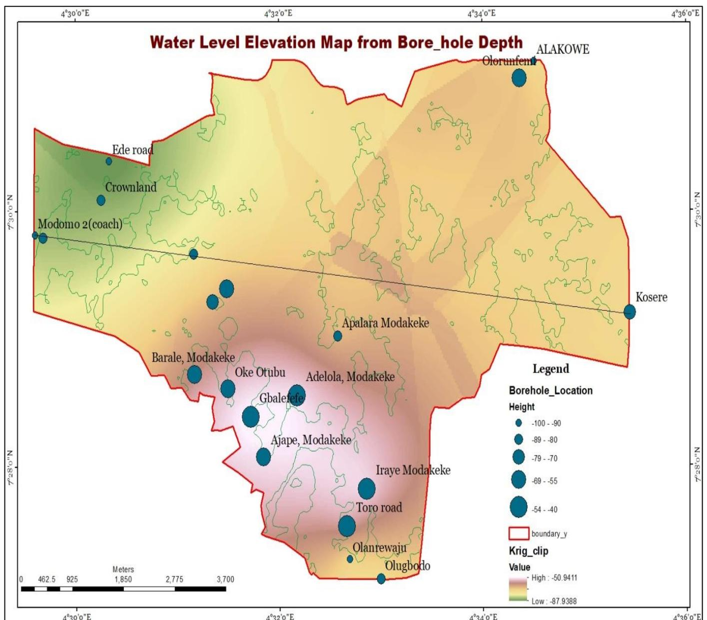
Fig 7 Water Level Map Deduced from Bore Hole Depth
