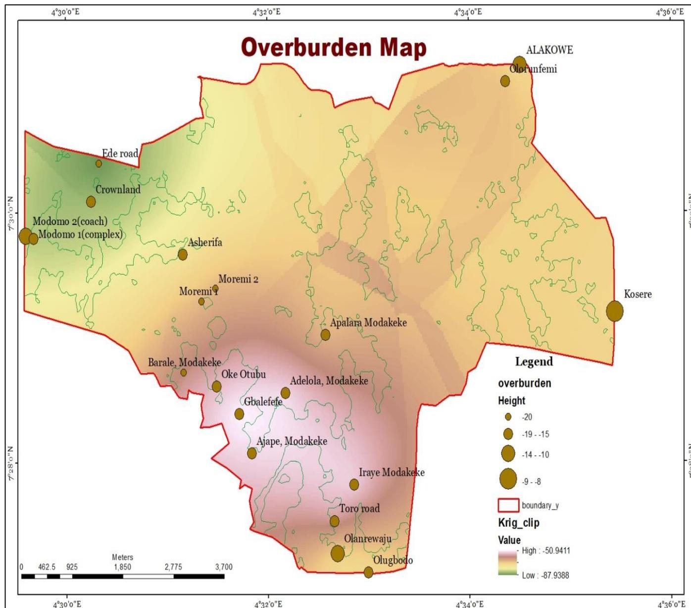
Fig 11 Showing Borehole Overburden from Selected Bore-Hole Locations as Soil Test for the Area
