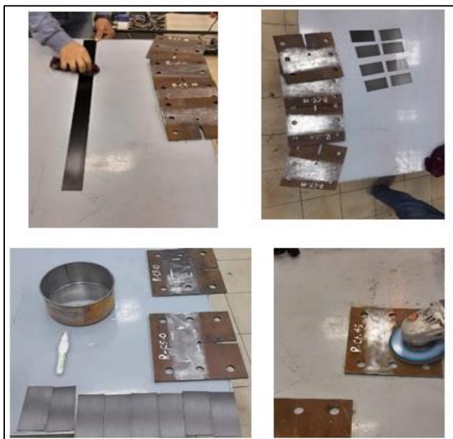
Fig 3 Preparing and Cutting CFRP Laminates
