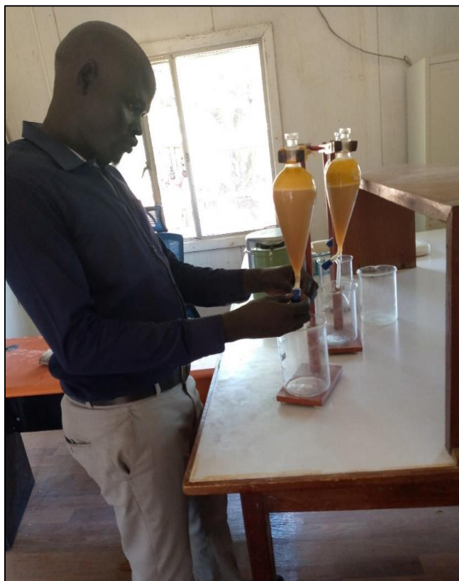
Fig 5 Separation of Oil from Water after Boiling (Photo by Deng Manyang Anyieth)
