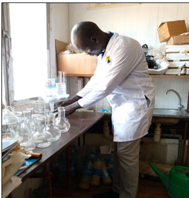
Fig 2 Filtration of Ash Solution in Progress (Photo by Daniel Majur Dum)
