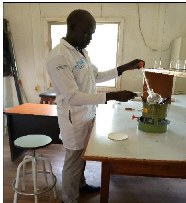
Fig 7 The Reaction between the Boiling oil and the Ash Filtrate as a Soap Production Step (Photo by Ajah Deng Neka)
