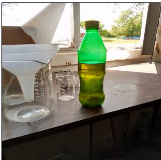
Fig 6 The Extracted Oil from the Seeds of Balanites aegyptiaca (Photo by Lin Yar Bol Riak)
