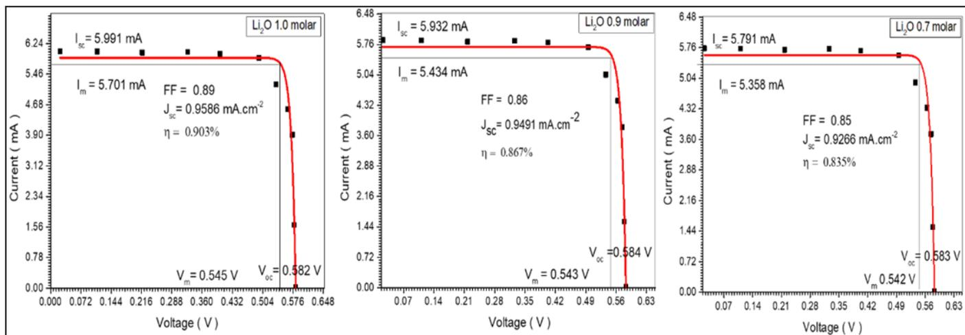
Fig (8) Current–Voltage (I–V) Characteristics of Li<sub>2</sub>O-Based Solar Cells at Different Concentrations (1.0 M, 0.9 M, 0.7 M)
