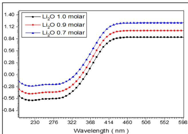
Fig 3 The Transmission of Li<sub>2</sub>O Thin Films
