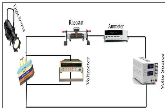
Fig 1 Schematic Diagram of IV Circuit of Thin Film Solar Cell.
