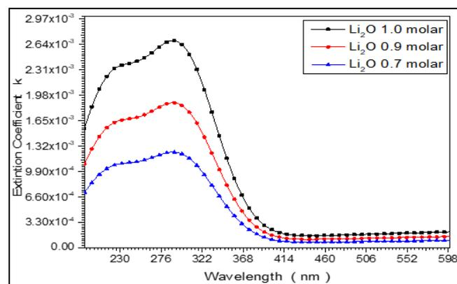
Fig 5 The Absorption Coefficient of Li<sub>2</sub>O Thin Films
