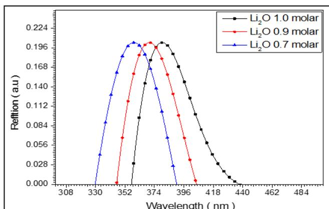
Fig 4 The Reflection of Li<sub>2</sub>O Thin Films
