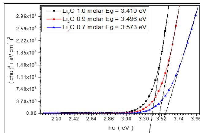
Fig 7 Optical Band Gap ( $E_g$ ) of  $\text{Li}_2\text{O}$  Thin Films
