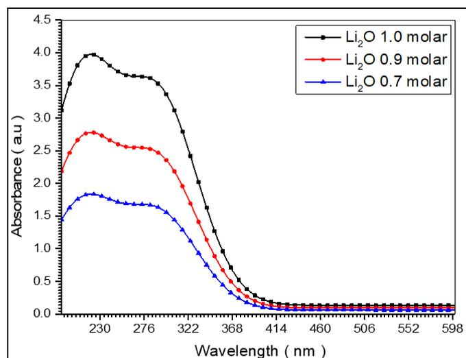
Fig 2 The Absorbance of  $\text{Li}_2\text{O}$  Thin Films
