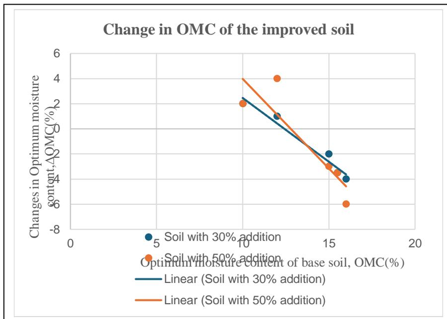
Fig 2: Variation in OMC of Base Soils for Recycled Aggregate Addition
