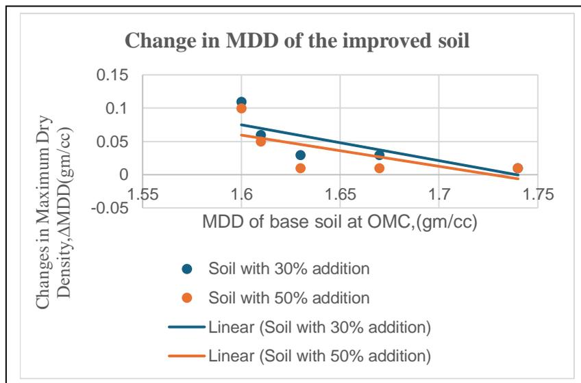
Fig 3: Variation in MDD of Base Soils for Recycled Aggregate Addition
