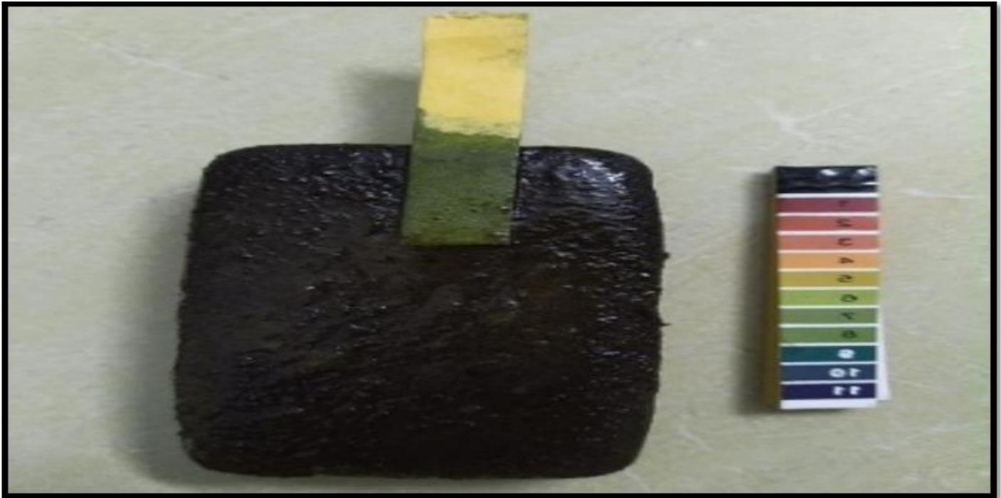
Fig 2 pH Determination
