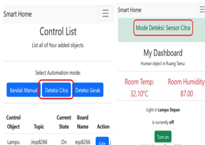
Fig. 16: Selecting the image sensor detection mode and a message indicating that the mode is active
