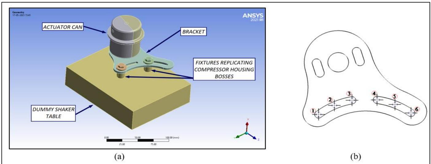
Fig 4 (a) Geometry Setup Detail from ANSYS Mechanical, (b) Mounting Positions on Bracket
