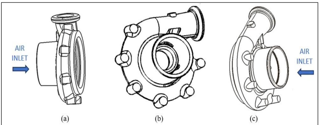
Fig 2 (a) Bearing Housing Side, (b) Outer Side, (c) Air Inlet Side
