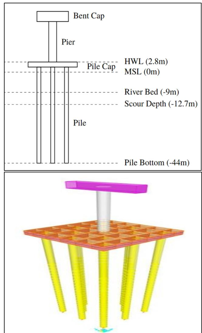
Fig 1 Elevation view and 3D Model of Bridge Substructure
