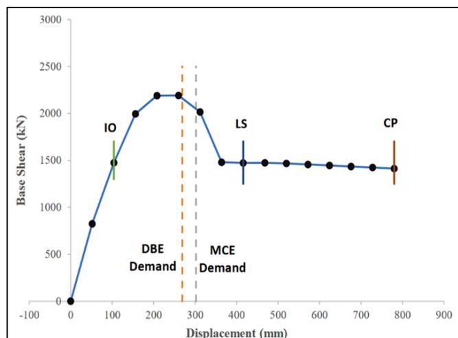
Fig 3 Pushover Curve with Capacity and Demand
