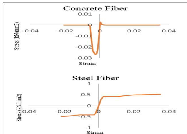
Fig 4 Stress-Strain Curve of Concrete and Steel Fiber
