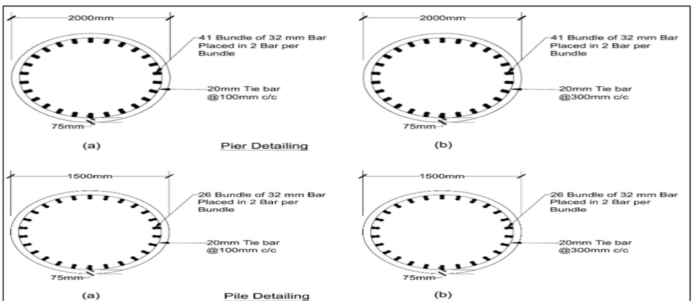
Fig 2 Cross Section Detailing of Pier and Pile (a) Confined Region, (b) Unconfined Region
